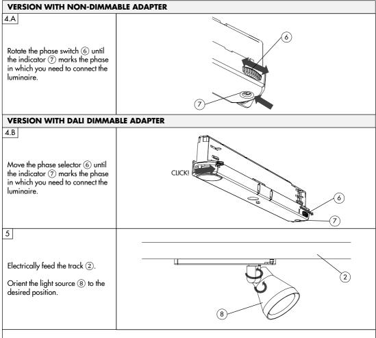
**NOTE**: To move the luminaire on the electrified track or to change the phase, previously make sure that the track has not network voltage.
